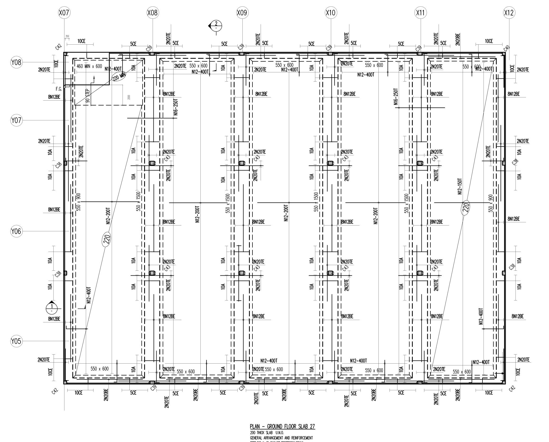
REFER DWG. No GR-27.02 FOR PRESTRESSING DETAILS. SLAB AND SLAB BAND THICKNESSES SHOWN ON PLAN ARE CONSTANT. REFER ARCHITECTS DRAWINGS FOR SLAB FALLS, KERBS, DRIP GROOVES AND ALL NON-
